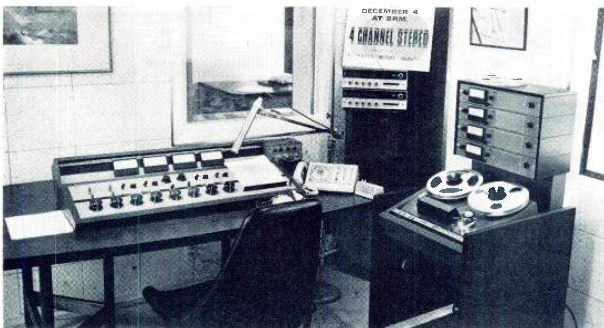
Homemade quad board at K-101 and special Ampex 1/2-inch quad machine originate quadcasts in Bay Area.
